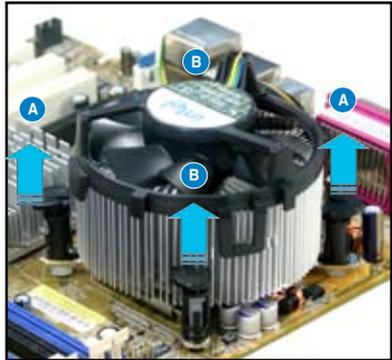
4. Carefully remove the heatsink and fan assembly from the motherboard.
