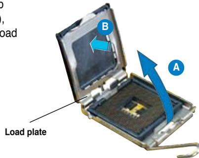
5. Position the CPU over the socket, making sure that the gold triangle is on the bottom-left corner of the socket. The socket alignment key should fit into the CPU notch.
