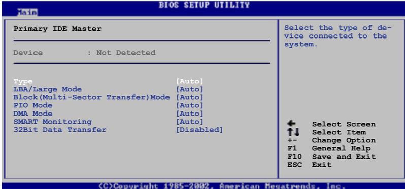
The BIOS automatically detects the values opposite the dimmed items (Device, Vendor, Size, LBA Mode, Block Mode, PIO Mode, Async DMA, Ultra DMA, and SMART monitoring). These values are not user-configurable. These items show Not Detected if no IDE device is installed in the system.
