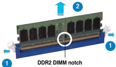
2. Remove the DIMM from the socket.
