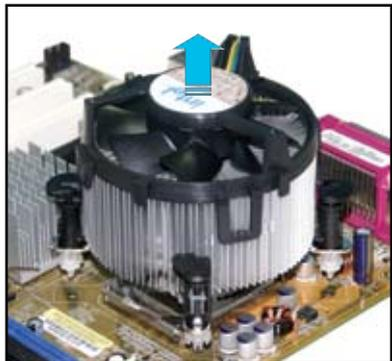
5. Rotate each fastener clockwise to ensure correct orientation when reinstalling.
